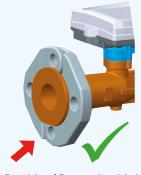
The flat side of flange should show be oriented to the counter flange.
