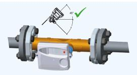
» Align the flow meter in the correct position (electronics ± 45° from horizontal position).
